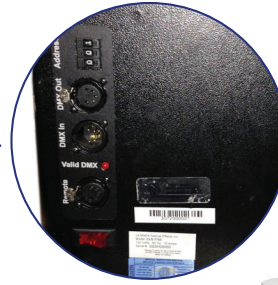
Built in 5-Pin DMX control for Fan & Flow Settings
