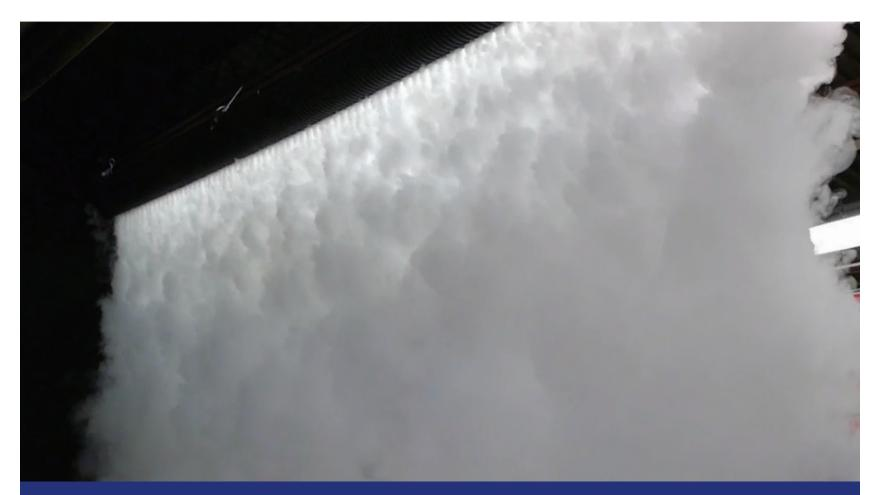
The Fog Curtain is designed to be used in conjunction with one of our low fog systems (low fog generator and a fog machine) such as the Eclipse. The combination of these machines can create a dramatic waterfall effect, sending fog cascading to the stage.
